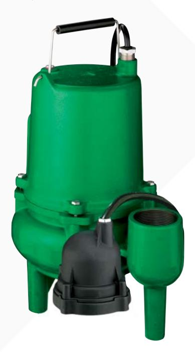
The Myers MSP50 submersible pump is specifically designed to meet the demands of handling wastewater and sewage in residential and commercial building applications. The 2 inch NPT discharge pump (3 inch discharge optional) is available with a powerful 1/2 horsepower motor, in both automatic and manual configurations; and can handle capacities up to 150 gallons per minute and heads to 29 feet.
